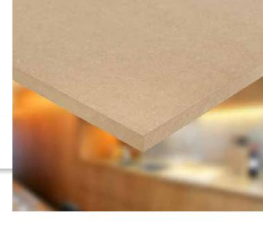
Firax Hydro® Pure also meets the criteria required for the MR50/grade 135 designation (ANSI A208.2-2016). It passes the 24-hour submersion test (MR10) and the 6 cycle accelerated aging test (MR30).
